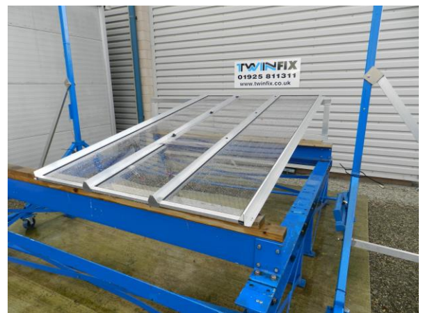
Below: Testing the hatch to the non-fragile drop test, where it passed with a 'B' designation, the highest that can be achieved with any polycarbonate glazing
