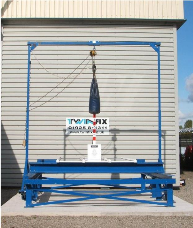
The Advisory Committee for Roofwork, led by the Health & Safety Executive, undertook research that led to the development of this test, which represents an impact on a roof surface. Twinfix has undertaken the required multiple drop tests on to the Multi-Link-Panel NF, achieving a 'B' rating.
