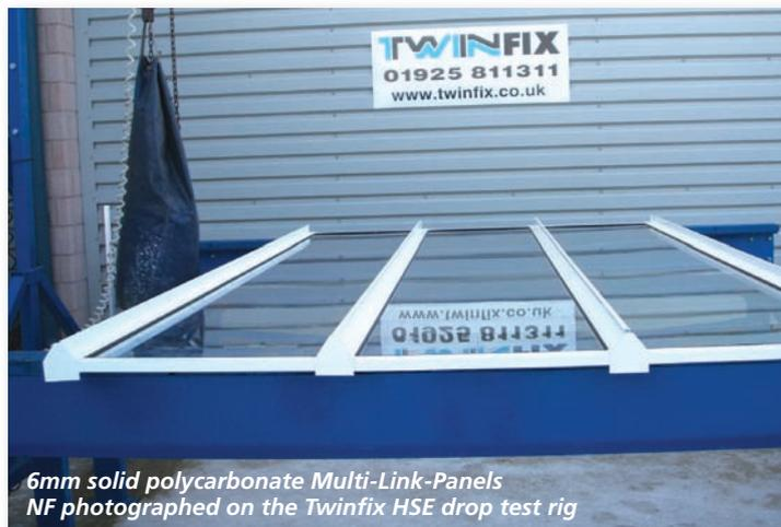
hold this material – the drop bag causes the multiwall sheet to flex out of the glazing bars and the drop bag falls through the resulting hole. 16mm multiwall polycarbonate fitted into a glazing bar **fails** the test.
